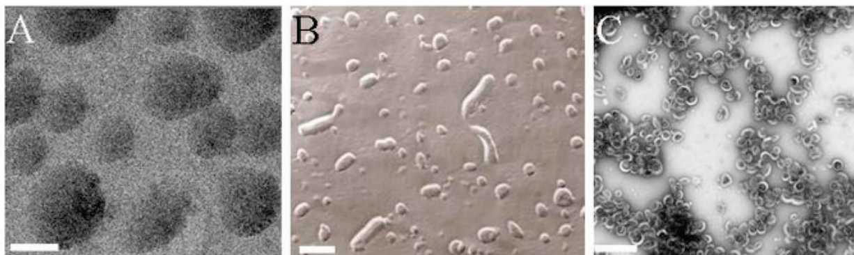
Figure 1. (A) Cryo-EM image showing the solid, dense spherical structures obtained upon self-assembly of AF-1 monomers at an elevated temperature of 70 °C; scale bar = 100 nm. (B) Freeze-fracture micrograph (scale bar = 200 nm) and (C) transmission electron micrograph (scale bar = 500 nm) confirm the spherical morphology of the buckysomes in panel A and also indicate a similar size profile. All three images were obtained from the same buckysome sample.
